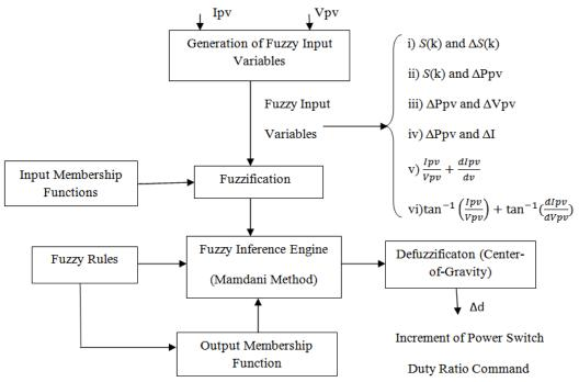
Figure 4. Flow diagram of Fuzzy Controller
