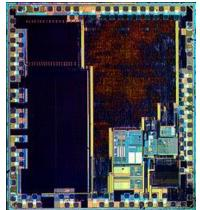
Figure 7. STM32F100C4T6B ARM Cortex-M3 microcontroller
