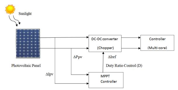
Figure 2. Solar Power with Maximum Power Tracking System
