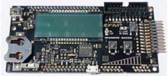
Figure 6. Energy Micro Wonder Gecko STK Board with EFM32WG990
