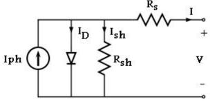
Figure 1. Equivalent Circuit diagram of PV cell
